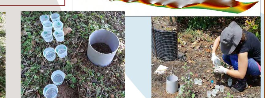
4. Monitoring of soil erosion and deposition rates (silt fences, reference iron sticks, soil profile)
