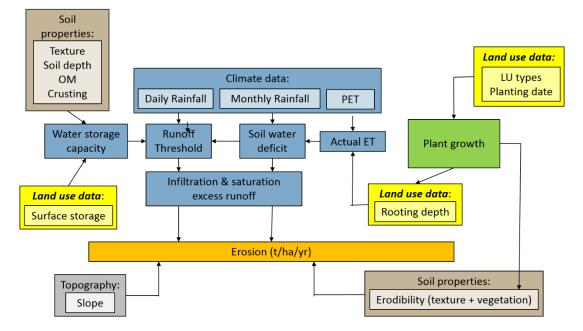
Figure 2.3: Schematic overview of processes in the biophysical model component
