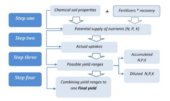
Figure 2.4: The four steps in the simulation procedure of QUEFTS (Source: Sattari et al., 2014).
