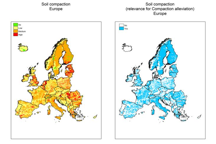
Figure 3.25: Relevance map for compaction (right) based on a compaction risk map for Europe. Medium and high categories on the compaction risk map are classified as relevant for compaction alleviation.
