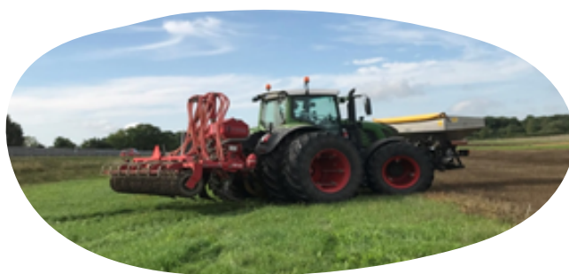
Sub tiller machinery used in Sweden for alleviating soil compaction
